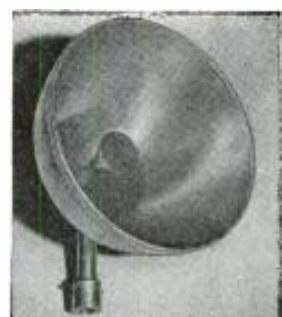
These u.h.f. energy directors are used with the Microtherm for various methods of therapy.
