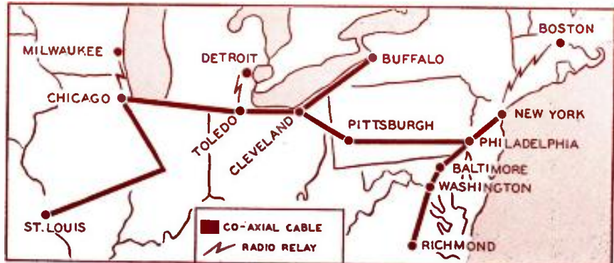
Eleven cities are now served by co-axial cables. Three more are connected to net by relays.
