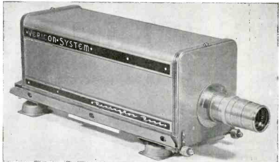
Fig. 1—The Vericon camera is the eye of the office or factory wired-television system.
