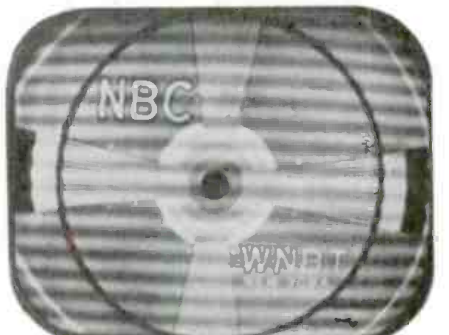
20. Horizontal lines of varying intensity.
