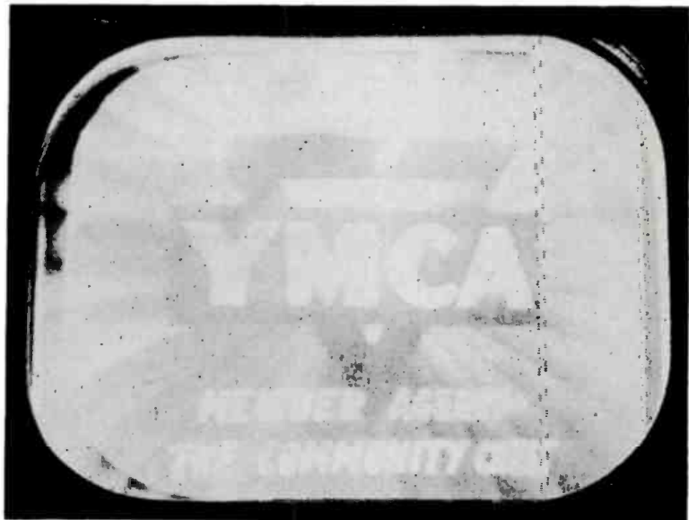
The antenna feeding this set was first installed in the handiest spot. Note light picture.
